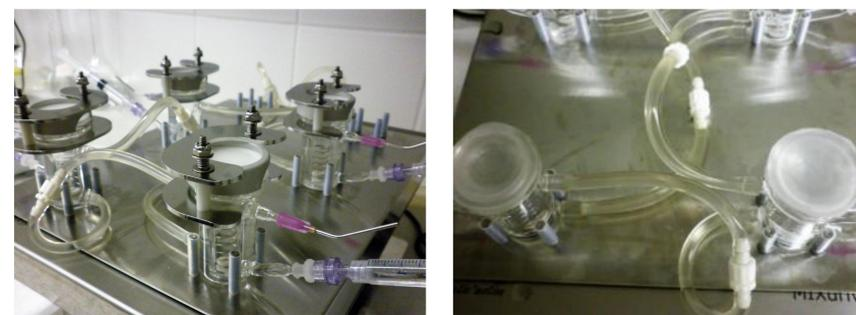
**Figure 5** (A-B) Franz diffusion cell instrumentation for *in vitro* permeation study
